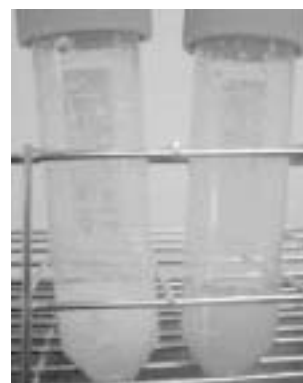
Fig. 5 Before and after the reaction of paper manufacture grime and industrial enzyme. The right is after reaction and the left is before.
