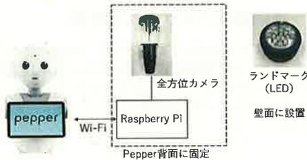
Fig.5 The composition of the Pepper's autonomous moving system
